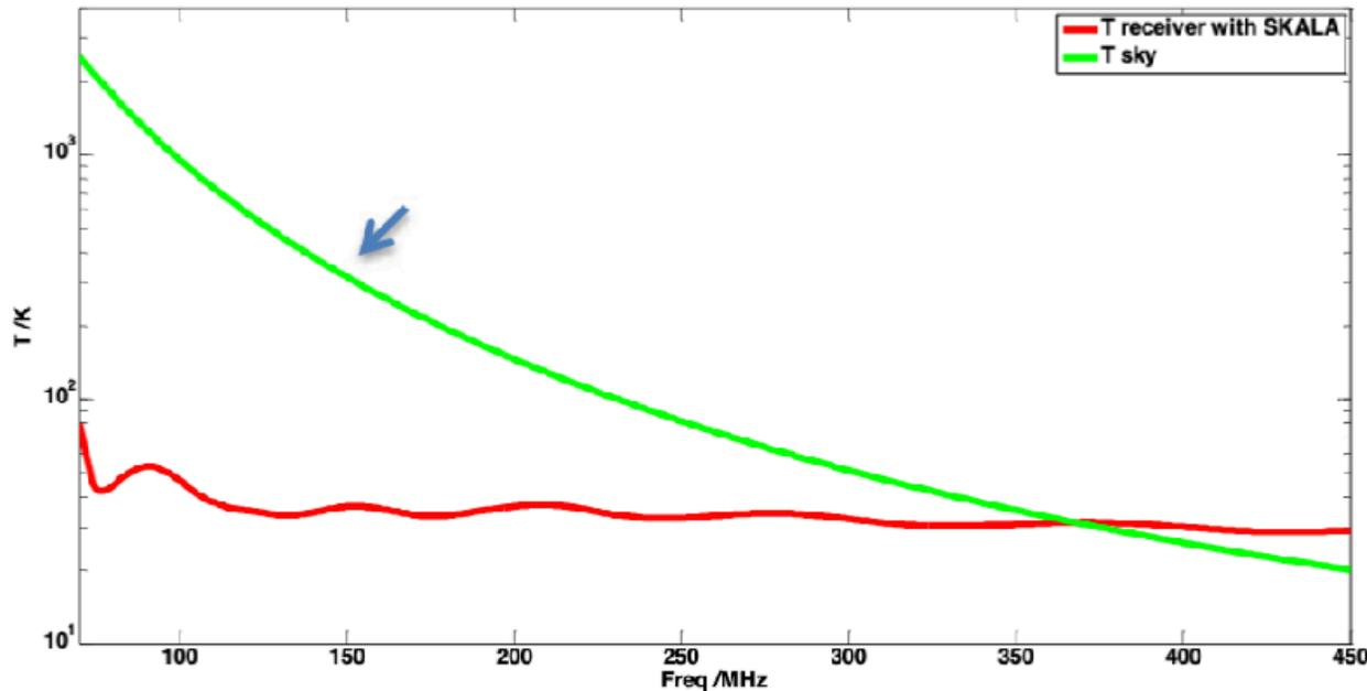
Fig. 9. Receiver noise temperature versus sky noise.
